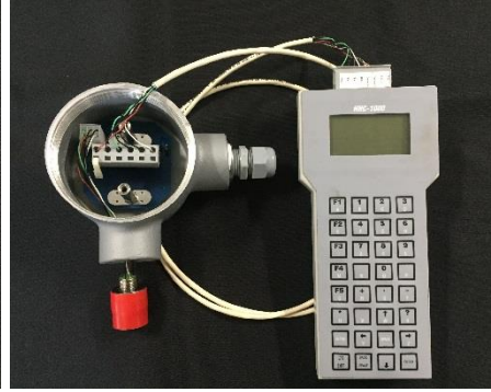
(HHC-1000 > Standard HHC Cable > Standard Sensor)
