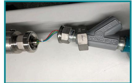
**9** Remove lower section of the 1" union and secure it to the sensor threads.
