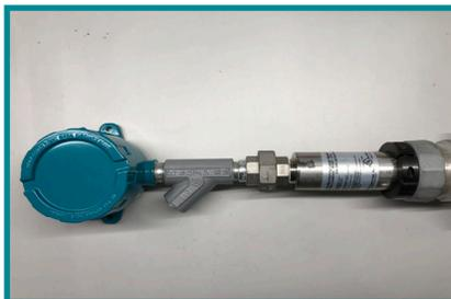
Join the 2110EX housing's 1" union with the top plug of the sensor, ensuring no wires are clipped in the process. Tighten to secure.
