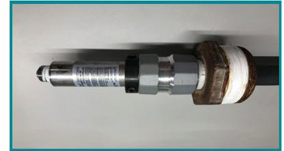
**5** Loosen the nut that is atop the 1" union of the 2110EX housing.
