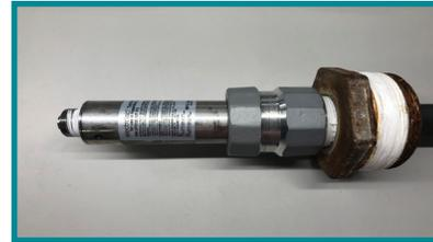
**4** Slide the black, oxide shaft collar onto the steel sleeve of the sensor. Secure directly above the cord grip/reducer.
