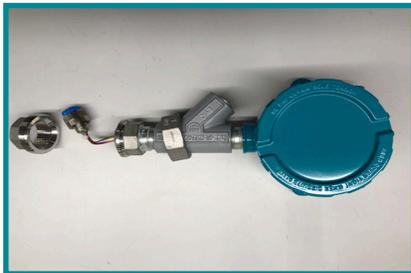
**6** Confirm that the number of connector pins on the sensor is compatible with the number of connector pins of the 2110EX housing.
