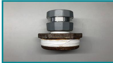
**3** Remove the ground screw from the sleeve of the sensor. Slide the cord grip/reducer onto the sleeve, 1' from the top of the sensor.
