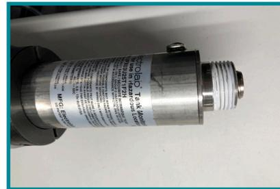
**8** Hold the 2110EX over the top of the sensor. Screw circular connector onto the connector of the top plug.
