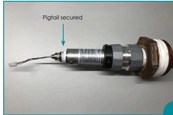
Apply thread sealant to the threads of the sensor flange. Remove the pigtail from the housing and connect the rounded end to the top of the sensor flange.
