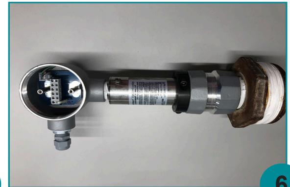
Tighten the housing onto the sensor flange. Feed the pigtail through the 1-inch port of the housing. Do NOT allow the wires to twist as the housing is screwed on. Connect the white end of the pigtail into the fuseboard. Place lid on housing. Sensor is ready for communications test and installation.
