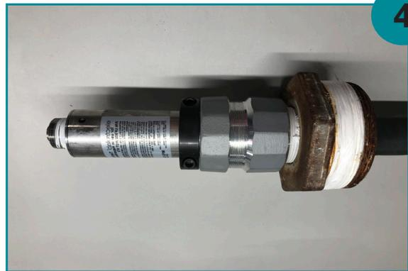
Slide the black, oxide shaft collar onto the stainless steel sleeve of the sensor above the cord grip/reducer bushing assembly. Tighten the side bolts of the shaft collar to prevent slipping. Replace the ground screw.
