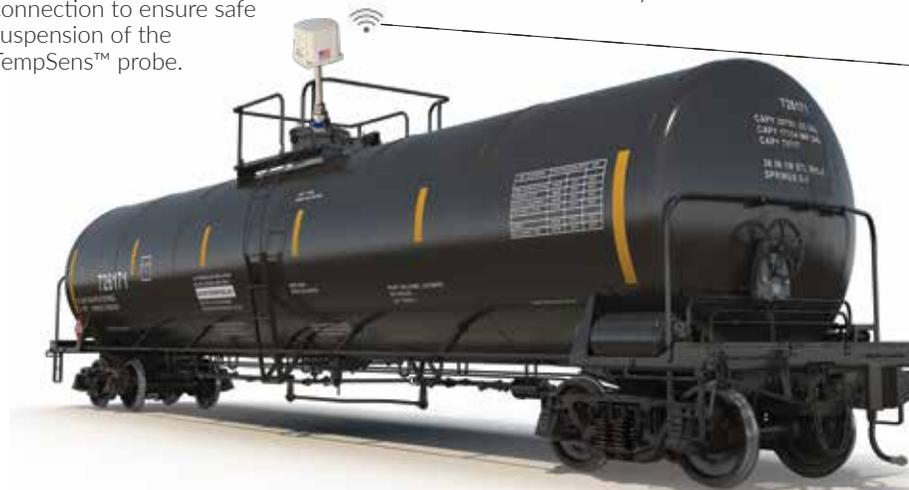
Electrolab's TankChek (optional) acts as a Modbus snooper on the communications line to display temperatures locally at ground level by the rail car. TankChek is hardwired to the wireless gateway.
